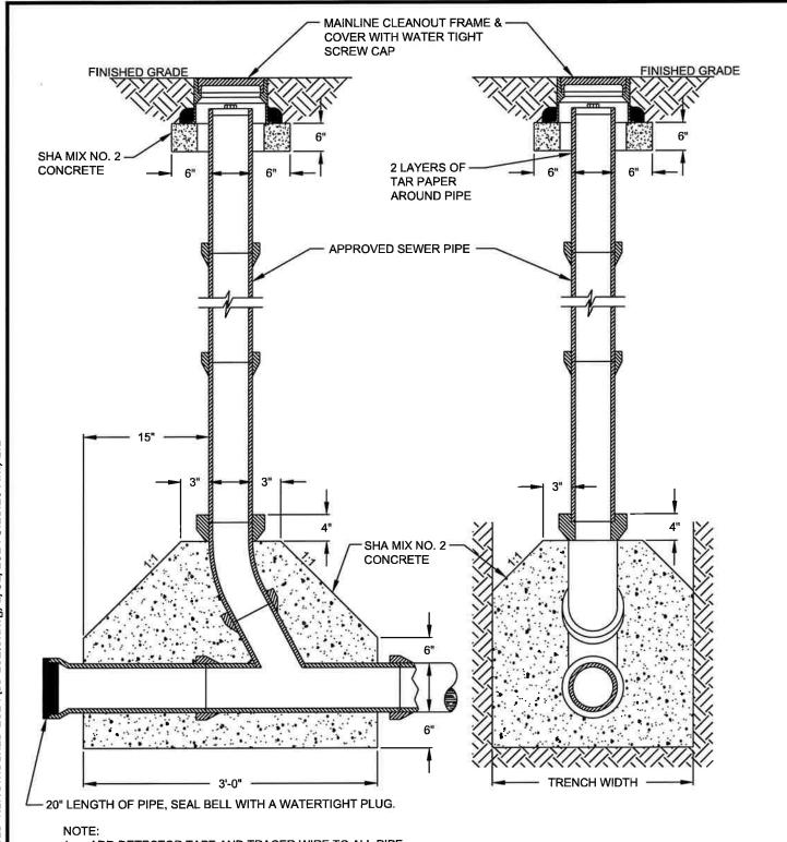
1. ADD DETECTOR TAPE AND TRACER WIRE TO ALL PIPE.
