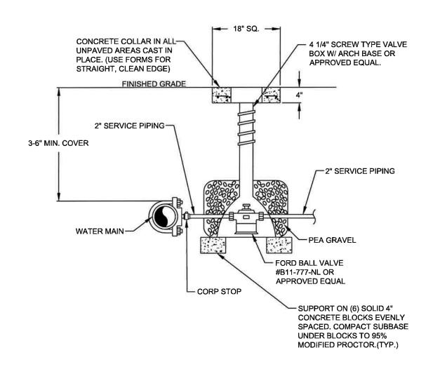
NOTE: VALVE BOX SHALL BE A 4  $\frac{1}{4}$ " PLASTIC VALVE BOX; MODEL P4B BY BINGHAM AND TAYLOR OR AN APPROVED EQUAL.
